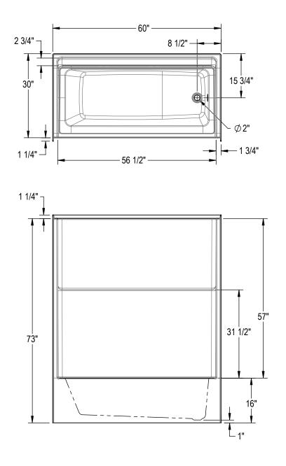
All dimensions are approximate. Structure measurments must be verified against the unit to ensure proper fit.
