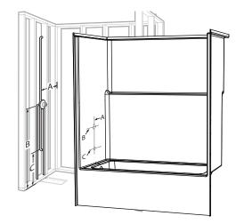
If mounting fittings — from stable reference points (back wall studs, floor) measure the locations of spout and valves. Note measurements below. For showers, refer to Diagram 2A; for tub-showers, refer to Diagram 2B.
