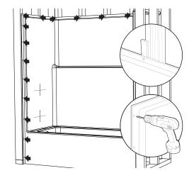
Pre-drill pilot holes. Fasten panel to framing at every stud and eight inches vertically through nailing flange.
