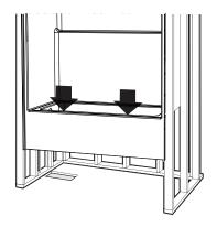
Place the unit into framing with drain fitting over and onto waste pipe with skirt firmly on the floor.
