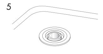
Assure waste pipe protrudes well into drain fitting. Maintain proper floor slope towards drain.
