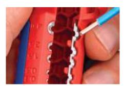
Stripping single conductor wire
