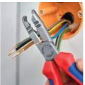
Cutting when shortening single conductors
