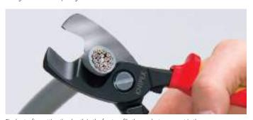
Final cut: after cutting the sheath in the front profile the conductors are cut in the rear area.
