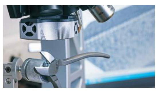
Shape and roughness of the diagonal cutter's cutting edge are precisely measured with an optical 3D measuring system.
