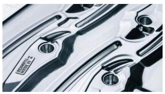
Forging die for the high leverage diagonal cutters with forged-in axle.
