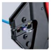
97 43 200 with crimping dies 97 49 06 for insulated terminals, plug connectors and butt
