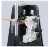
Precise, complete clean cut of the insulation
