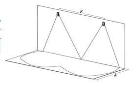
Note: Photometric results shown are based on a simulation using the AGI32 software with a 1 foot-candle average and 0.1 foot-candle minimum with a 40:1 maximum ratio. Thomas & Betts assumes no responsibility for local requirements or specific project variable. This is a guideline to be used as a design aid, not guarantee of any code compliance.
