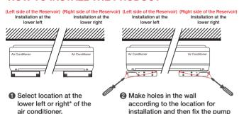
\*The product is configured out of the box for installation at the lower right. When installing on the left, move the rubber gaskets to the opposite side as shown in the figure, assemble it, and then install it so that the location of the reservoir is on the left.
