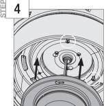
Align the keyhole slots in the light kit housing with the two screws. Make sure all the wires from the fan and the light kit are snug inside the center of the light kit, not pinched in between the upper switch housing and the light kit or hanging out of the sides.
