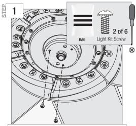
Partially install two light kit screws, found in the hardware bag, halfway into the motor housing as shown. It does not matter which two screw holes you choose.
