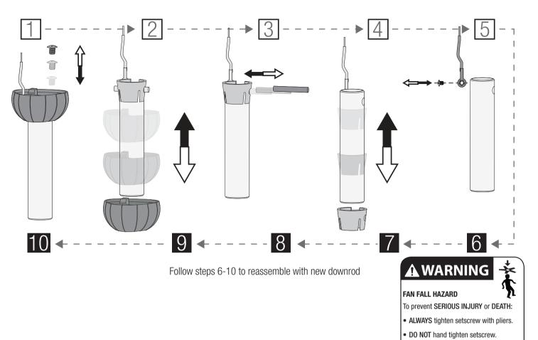
CHECK the setscrew is tight using pliers each time you change fan direction.
