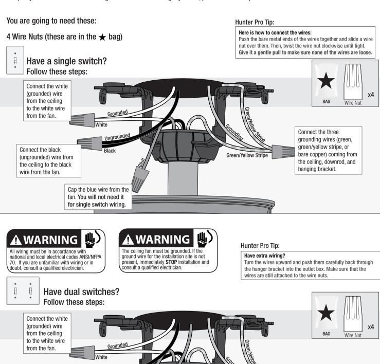
Connect the three grounding wires (green, green/yellow stripe, or bare copper) coming from the ceiling, downrod, and hanging bracket.
