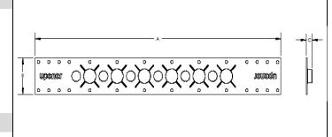
The PEX Wall Support Bracket provides rigid straight-through support for  $\frac{1}{2}$ " or  $\frac{3}{4}$ " AQUAPEX<sup>®</sup> tubing, fixed 2" on-center spacing, and allows the  $\frac{1}{2}$ " Plastic Bend Support (A5250500) to snap into place for  $\frac{1}{2}$ " AQUAPEX tubing as it exits the wall.
