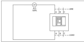
Warning: Never pass test current through an unterminated Neutral Sensor. Permanent sensor damage may occur if operated in this manner.
