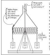
Lashing Instructions to 100,000A Maximum To comply with UL short circuit withstand ratings the adjacent Ø & N connections shall be lashed per the instructions provided below.
