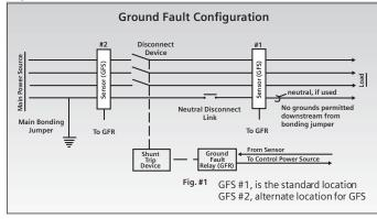
WARNING: The following should be performed only by qualified personnel as defined in NEC article 100. The ground fault sensor (GFS), ground fault relay (GFR), must be installed as in Figure 15. Note: Test report and test record forms found on Page 18 and 19 of this manual can be used to record ground fault field testing.
