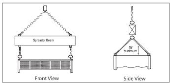
**3.4.2 Multi-section lifting** – The method of lifting a multisection unit is similar to lifting single section. The cables need to be connected to all lifting brackets. The lifting cables must have correct spreader from side to side (See Fig #1B). A crane with sufficient height and lift is required.
