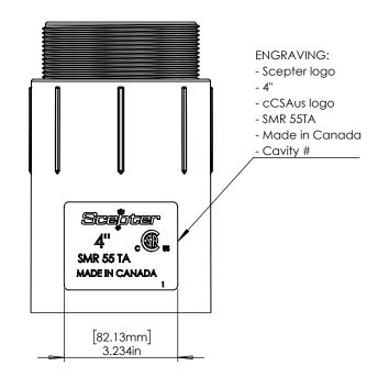
SIZES SHOWN ARE FOR REFERENCE 3D MODEL IS TO BE USED FOR MANUFACTURING / VERIFICATION
