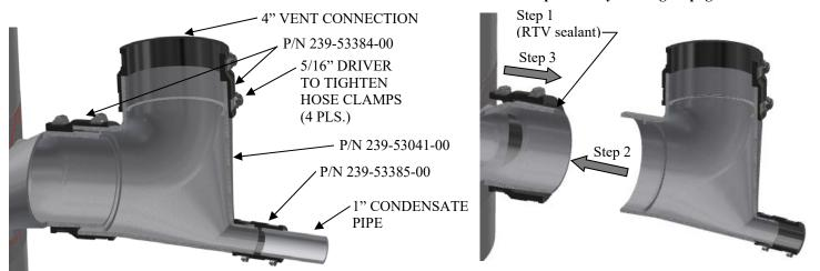
Apply clear RTV sealant around the entire circumference of the male end of exhaust pipe before installing the female end of the condensate elbow as shown above. Then pull forward vent adapter, p/n 239-53384-00 and tighten hose clamps to ensure no leaks.
