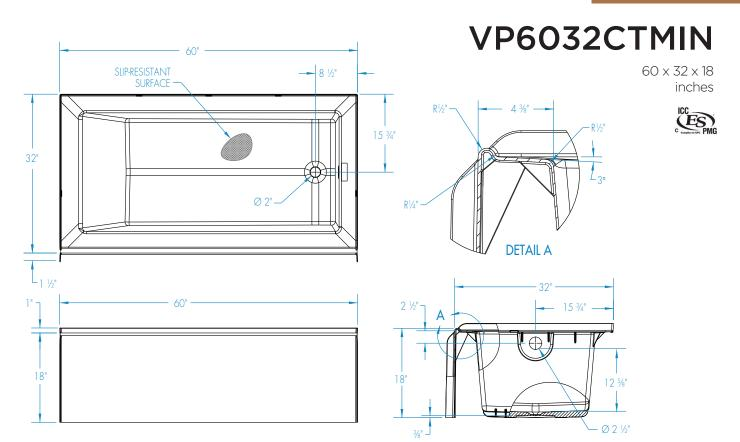
FEATURES Dimensional Tolerance ± 3/8". Dimensions needed for site preparation should be measured from the unit. Manufacturer assumes no responsibility for preparatory work.
