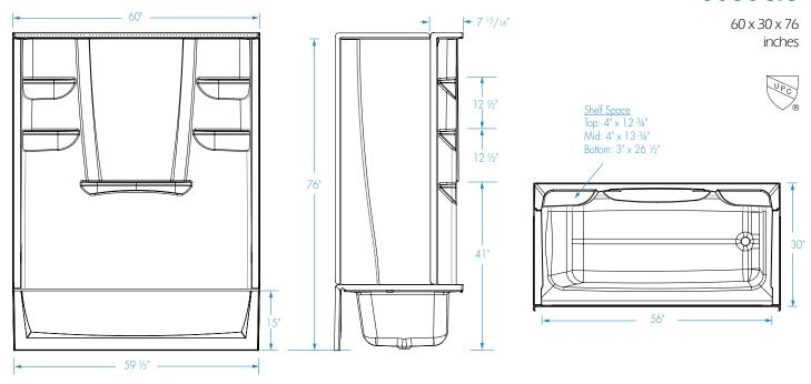
Assembled Model Components: 6030CTL (Base) or 6030CTR (Base), 6062CBW (Back Wall), 2462CSW (Side Walls)
