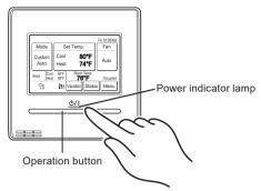
The Power indicator lamp remains lit while the indoor unit is operating.
