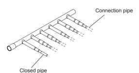
5. Place the Header horizontally so that the refrigerant separates evenly. They cannot be used vertically.
