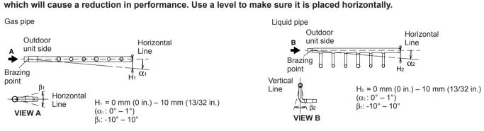
• During piping work, apply nitrogen gas while brazing the pipes. If pipes are brazed without applying nitrogen gas, it will create a large amount of evidation film, which will cause a critical malfunction.
