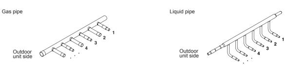
4. Install the supplied closed pipes to the header outlets that will remain unused.
