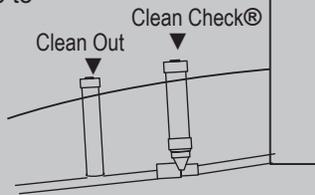
have this valve checked periodically to insure that it is operating properly. Under normal installation and use, a three month inspection interval is recommended. It is also recommended that a licensed plumber perform these inspections.
