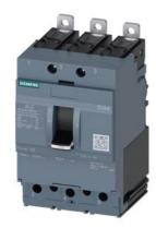
circuit breaker 3VA4 UL frame 125 breaking capacity class S 25kA @ 480 V 3-pole, line protection TM210, FTFM, In=30A overload protection Ir=30A fixed short-circuit protection Ii=10 x In clamp connection
