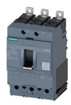
circuit breaker 3VA4 UL frame 125 breaking capacity class S 25kA @ 480 V 3-pole, line protection TM210, FTFM, In=125A overload protection Ir=125A fixed short-circuit protection Ii=10 x In clamp connection
