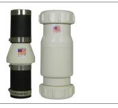
Rubber Hose Coupling: Valves are designed to fit on standard sump pump line connections. Easy to install over 1 1/2" or 1 1/4" PVC pipe (schedule 40 & 80), steel pipe, or copper tubing. One piece housing construction, no gasket to fail or leak. Housing is made of high grade ABS plastic, clamps are 301 stainless steel, and hoses are SBR rubber. Valve body will glue up to standard PVC pipe & fittings for installation options. Non-metallic and cannot corrode. Color is red/black.
