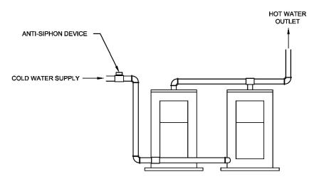
Figure 3 (Dual Water Heater Installation)
