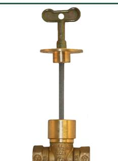
The C-67 AGA Gas Valve is for use on any gas fireplace or appliance. Using the included operating rod, the installer can install the valve from 1" to 14" depth, allowing it to be installed "below-the-joist," eliminating fittings and installation time. The C-67 Gas Valve is also used as a shutoff for any gas burning appliance.
