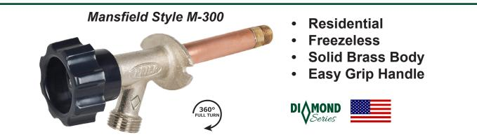
PRIER 300 Series provides a year round source of water to areas of structures that are subject to freezing temperatures. The hydrant valve is connected to the supply piping in the heated portion of the structure, eliminating the possibility of freezing.
