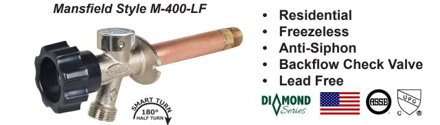
PRIER 400-LF Series is made with lead free brass and provides a year round source of water to areas of structures that are subject to freezing temperatures. The hydrant valve is connected to the supply piping in the heated portion of the structure, eliminating the possibility of freezing. The PRIER 400 Series features half-turn design for years of easy operation.
