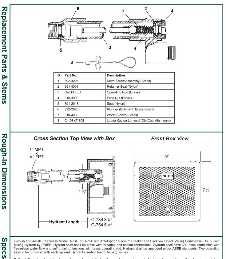
Optional: Furnish and install water box for each hydrant. Hydrant box shall be manufactured of solid cast brass with a polished brass or polished nickel bronze finish. Access to the water box shall be provided by the same operating key as the freezeless hydrant. \*4" to 24" in 2" increments.
