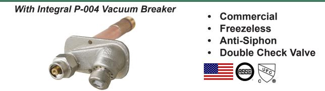
PRIER C-534 provides a year round source of water to areas of structures that are subject to freezing temperatures. The hydrant valve is connected to the supply piping in the heated portion of the structure, eliminating the possibility of freezing. To assure freeze protection, the hydrant will drain even with the hose attached and under pressure without sprayback!
