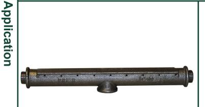
The C-69 Cast Iron Burner Bar is the original burner bar with ash shields to prevent clogging of the gas ports. The tee style design has three 1/2" I.P.S. tappings for gas service from bottom or either side. The burner bar is shipped with two plugs for the unused ports
