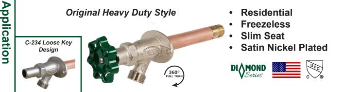
PRIER C-134 provides a year round source of water to areas of structures that are subject to freezing temperatures. The hydrant valve is connected to the supply piping in the heated portion of the structure, eliminating the possibility of freezing. Ordering the C-234 gives you the same style hydrant but with a vandal proof extended lockshield with operating key.
