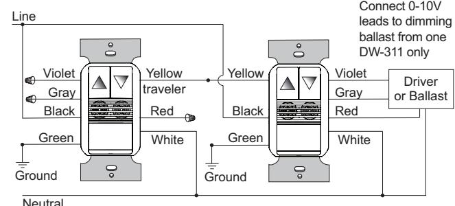
**WARNING:** Grounding the violet and gray wires can damage the unit. Do not apply power to the sensor until all wires are connected or capped off if the driver is to be installed at a future time.
