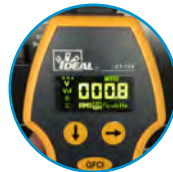
Displays neutral to ground voltage
