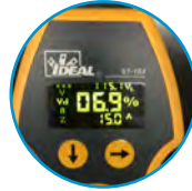
Displays Voltage Drop at 12, 15 & 20 Amps
