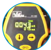
Trips GFCI at 6mA or 30mA
