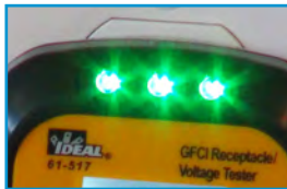
Green Lights Indicate Correct Wiring
