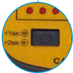
On/Off Button Confirms Tester is Working
