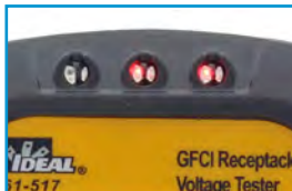
Red Lights Indicate Incorrect Wiring
