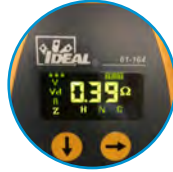
Displays Impedance of hot, neutral & ground
