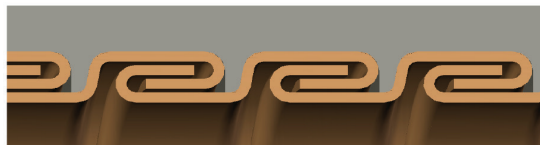
Interlocked Design 3/8" through 4"
