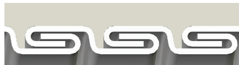
Interlocked Design 1-1/2" through 4"
