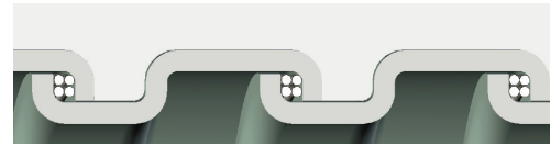
Square-Locked Design with cord packing 3/8" through 1-1/4"
