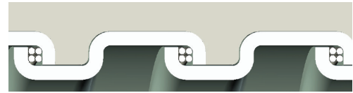
Square-Locked Design with cord packing 5/16" through 1-1/4"
