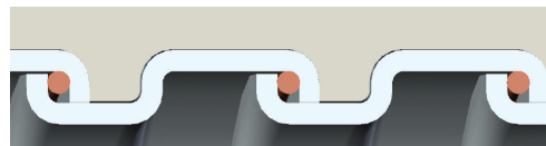
Square-Locked Design with integral bonding wire 3/8" through 1-1/4"
