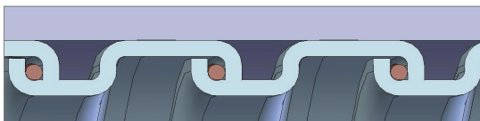
Square-Locked Design with integral bonding wire 1/2" through 1"
