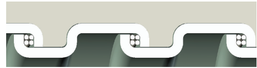
Square-Locked Design with cord packing 3/8" through 1-1/4"
