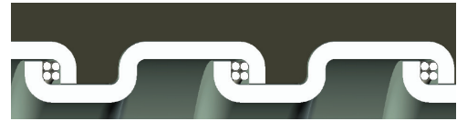
Square-Locked Design with cord packing 3/8" through 1-1/4"
