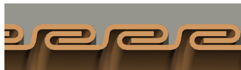
Interlocked Design 3/8" through 4"
