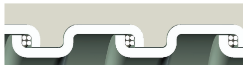
Square-Locked Design with cord packing 3/8" through 1-1/4"
