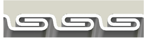
Interlocked Design 1-1/2" through 4"
