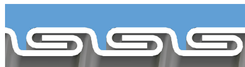
Interlocked Design 1-1/2" through 3" with no bonding wire
