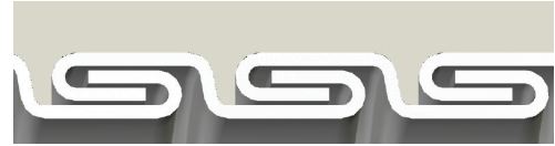
Interlocked Design 1/4" and 1-1/2" through 6"
