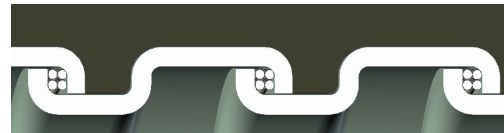
Square-Locked Design with cord packing 3/8" through 1-1/4"
