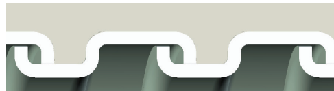
Square-Locked Design 3/8" through 2"
