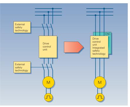
Fig. 5/1 External safety technology, integrated safety technology
