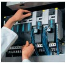
Fig. 6/7 Just like the I/O modules of the ET 200S, motor starters can also be replaced during production, which has a positive impact on increasing overall plant availability
