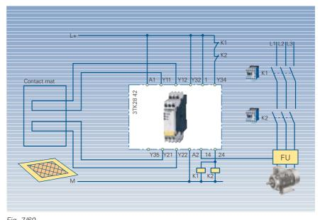
Fig. 7/60 SIGUARD 3TK2842, contact mat, Category 3 acc. to EN 954-1, 2-channel, autostart
