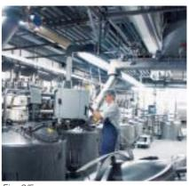
Fig. 6/5 The raw ingredients are transported to the mixing containers via the screw conveyor system controlled and safeguarded using ET 200S motor starters
