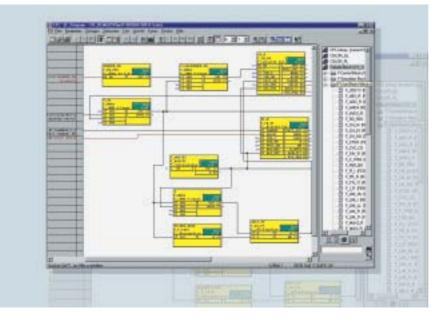
Fig.4/2 Graphic configuring of the S7-400/FH using the CFC Engineering Tool
