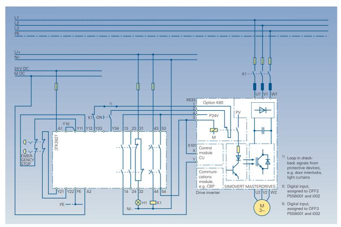
Fig. 7/94 Stop Category 1, 2-channel, with feedback circuit, Category 3 acc. to EN 954-1; Function where the motor is shut down along the torque limit in a controlled fashion.
