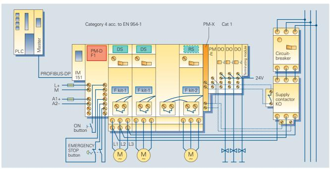
Fig. 7/91 EMERGENCY STOP circuit with integrated pneumatic valves
