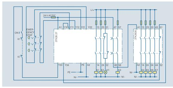
Fig. 7/19 3TK28 27 expanded by 3TK28 30 for EMERGENCY STOP, Category 4 (Category 3 for delayed contacts), two-channel, monitored start
