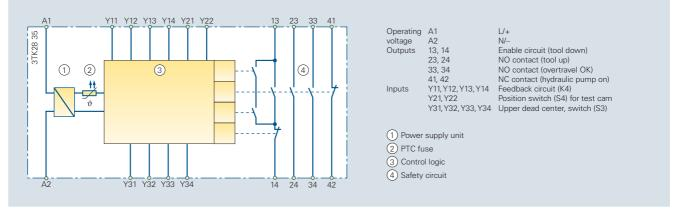
Fig. 7/36 Internal circuit diagram of the 3TK28 35 overtravel tester
