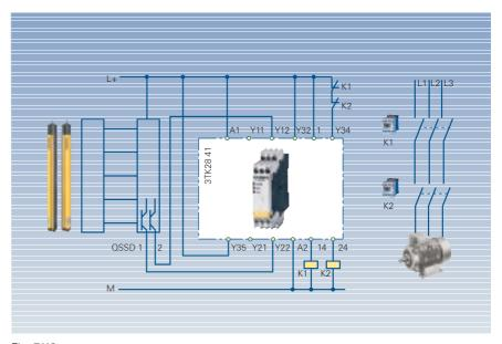
Fig. 7/49 SIGUARD 3TK2841, light grid monitoring, Category 4 acc. to EN 954-1, 2-channel, with feedback circuit, autostart
