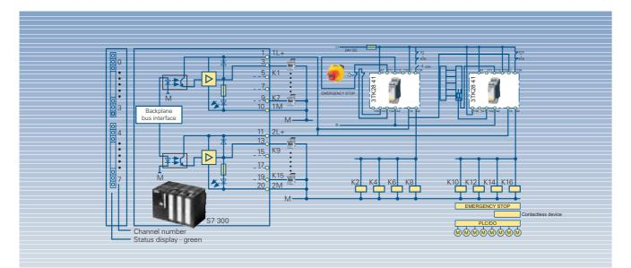
Fig. 7/53 SIGUARD 3TK2841, EMERGENCY STOP and light grid, Category 4 acc. to EN 954-1, cascaded with operational control of a standard PLC (SIMATIC S7 300/ET200M)
