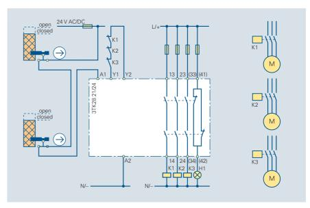
Fig. 7/23 3TK28 21/24 for protective door monitoring with tumbler (2 protective doors are cascad-ed, each with 2 SIGUARD position switches with tumbler) Category 2 acc. to EN 954-1, single-channel, with feedback circuit, outpotter. autostart
