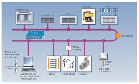
Fig.2/2 PROFIsafe and PROFIBUS nodes co-exist on the same cable
