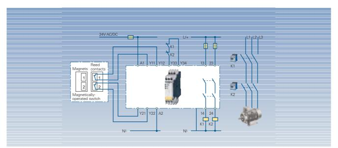
Fig. 7/31 Protective door monitoring with magnetically-operated switch, Category 3 acc. to EN 954-1, two-channel, with feedback circuit, autostart
