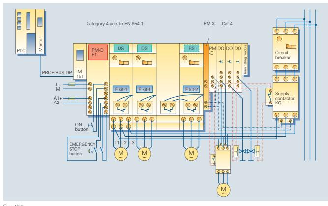
Fig. 7/92 EMERGENCY STOP circuit with integrated external actuators
