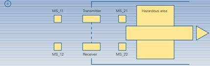
4. After one of the inputs for the muting sensors MS\_21 and MS\_22 = 0 (the product enables the sensors), the MUTING function is exited (Q = 1, MUTING = 0). The MUTING function may be active for a maximum time parameterized at the input TIME\_MAX.
