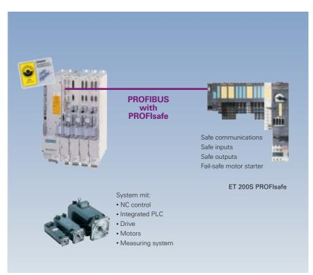
Fig. 5/24 Sensor-actuator integration through ET 200S PROFIsafe
