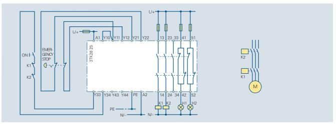
Fig. 7/14 3TK28 25 EMERGENCY STOP, Category 4, two-channel, according to EN 954-1, monitored start
