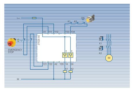
Fig. 7/43 SIGUARD 3TK28 40, basic electronic device, EMERGENCY STOP, 2-channel, Category 3 acc. to EN 954-1
