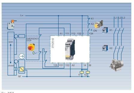
Fig. 7/57 SIGUARD 3TK2842, EMERGENCY STOP and protective door monitoring, Category 4 acc. to EN 954-1, 2-channel, with tumbler, monitored start
