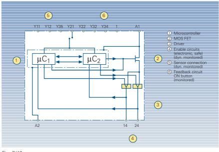
Fig. 7/42 SIGUARD 3TK28 41, internal circuit diagram, standard electronic device
