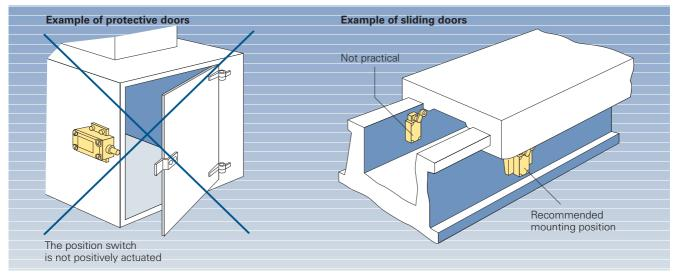
Fig. 3/22 Mounting position switches to ensure the correct function
