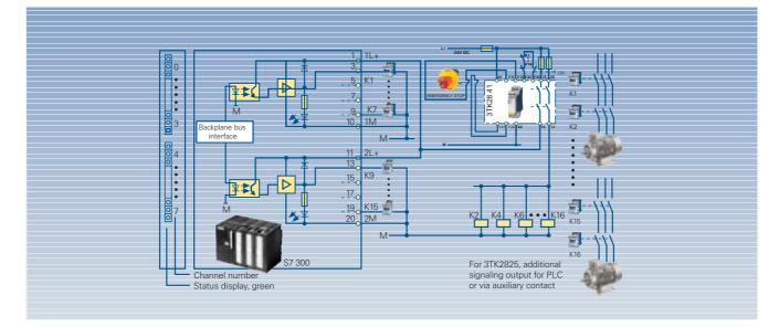
Fig. 7/20 EMERGENCY STOP, Category 4 acc. to EN954-1, 3TK2823(25) in conjunction with operational control of a standard PLC (SIMATIC S7-300/ET200M), load current for each enable circuit, max. 5 A. When using 3TK285.-.. max. 10 A for each enable circuit
