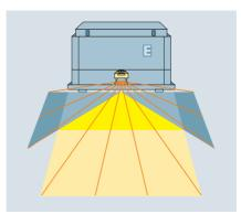
Fig. 3/55 Example - protecting hazardous areas using 4 protective fields which can be toggled between
