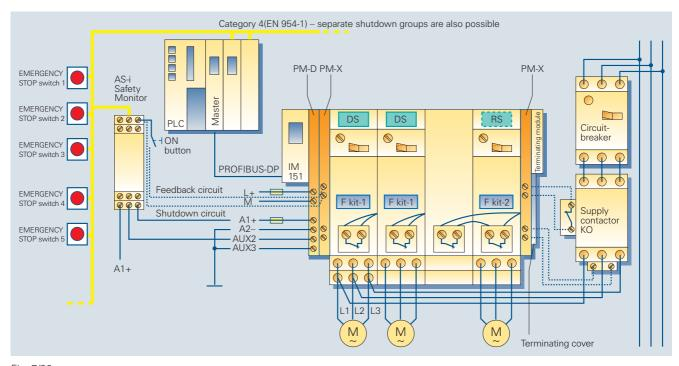
Fig. 7/90 SIMATIC ET 200S SIGUARD and AS-i Safety at Work
