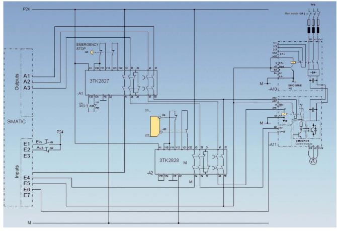
Fig. 7/95 EMERGENCY SWITCHING-OFF and EMERGENCY STOP, Stop Category 1 acc. to EN 60204, 2-channel with feedback circuit, control Category 3 acc. to EN 954-1
