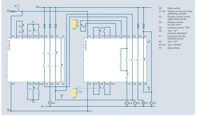
Fig. 7/37 3TK28 34 two-hand control device in conjunction with a 3TK28 35 overtravel tester to mon-itor the overtravel on linear hydraulic, pneumatic and spindle presses acc. to VBG 7 n 5.2 § 11, Category 4 acc. to EN 954-1
