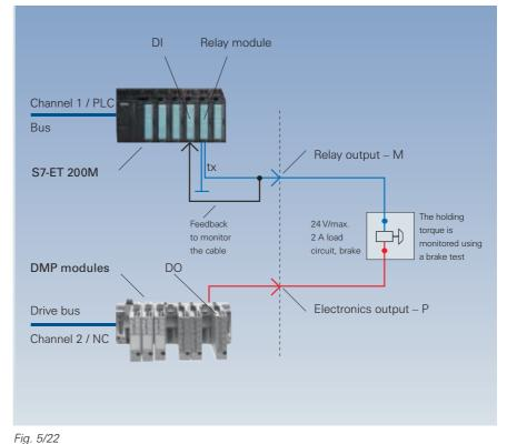
24 V load circuit – P/M switching – example of Safe brake Control
