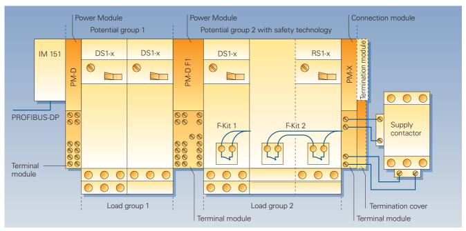
Fig. 3/67 Structure of a safety-related motor starter
