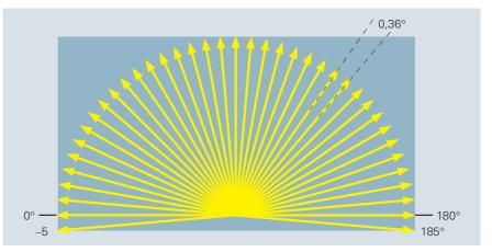
Fig. 3/53 Working area and angular resolution
