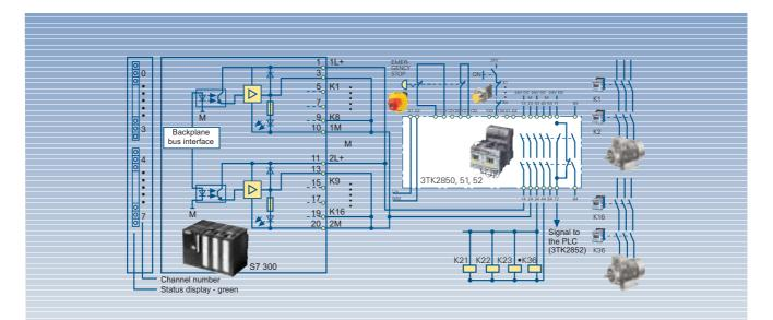
Fig. 7/67 3TK285.-.., EMERGENCY STOP, Category 4 acc. to EN 954-1, P-M switching in conjunction with operational control of a standard PLC (SIMATIC S7 300/ET200M), load current per enable circuit, 10 A
