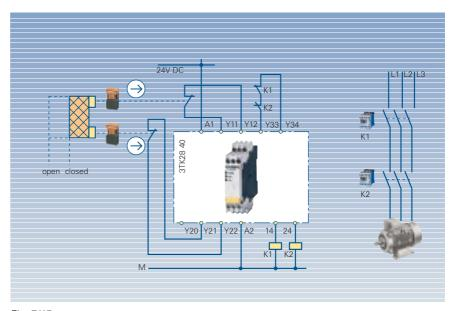
Fig. 7/45 SIGUARD 3TK2840, protective door monitoring, Category 3 acc. to EN 954-1, two-channel with feedback circuit
