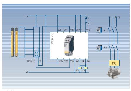
Fig. 7/59 SIGUARD 3TK2842, light grid monitoring, 2-channel, autostart, Category 4 acc. to EN 954-1
