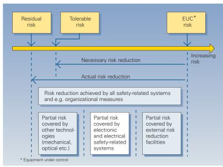
Fig. 1/13 Principle of risk reduction (acc. to IEC 61508)
