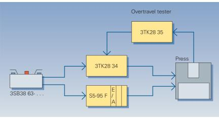
Fig. 3/14 Safety circuit of a two-hand control for presses
