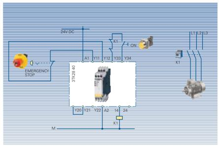
Fig. 7/44 SIGUARD 3TK2840, EMERGENCY STOP, Category 2 acc. to EN 954-1, single-channel, with feedback circuit
