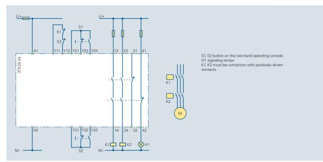
Fig. 7/35 3TK28 34 two-hand control device, Category 4 acc. to EN 954-1
