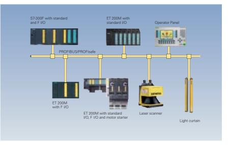
Fig. 4/7 Example of a configuration (F I/O is yellow, standard I/O is blue)
