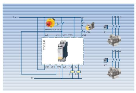
Fig. 7/47 SIGUARD 3TK2841, EMERGENCY STOP, Category 2 acc. to EN 954-1, one-channel, with feedback circuit, monitored start
