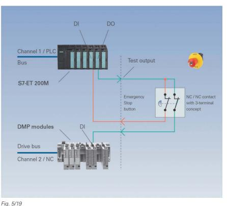
Sensor integration using the 3-terminal concept – example for Emergency Stop
