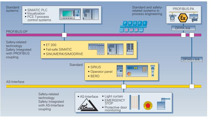
Fig. 2/1 The basic principle of "Safety Integrated": A unified automation system with integrated safety functions
