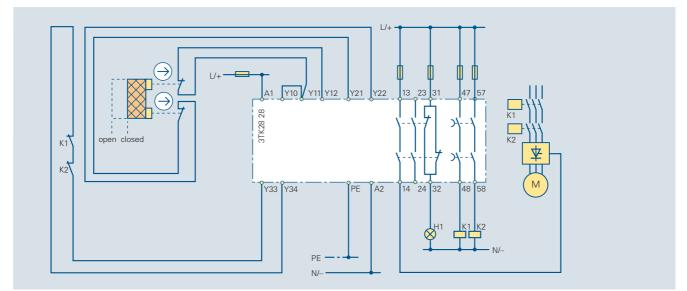
Fig. 7/29 3TK28 28 for protective door monitoring with 2 SIGUARD position switches, stop Category 1, Category 3 acc. to EN 954-1, two-channel, with feedback circuit, autostart
