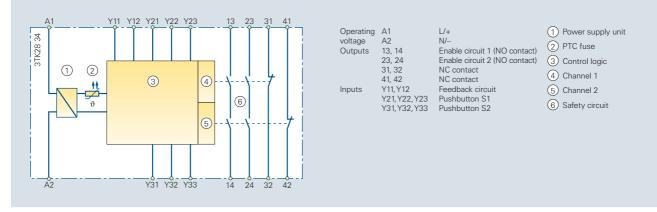
Fig. 7/34 Internal circuit diagram of the 3TK28 34 two-hand control device
