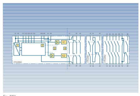
Fig. 7/61 SIGUARD 3TK2850, 51, 52, internal circuit diagram, electronic basic unit with auxiliary contactors, Category 3 acc. to EN 954-1
