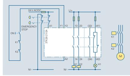
Fig. 7/11 3TK28 21/24 EMERGENCY STOP, Category 3 (4), two-channel with feedback circuit
