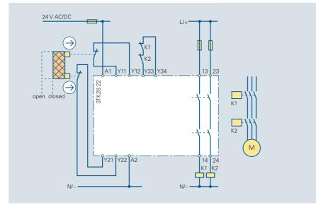
Fig. 7/25 3TK28 22 for protective door monitoring (protective doors, each with 2 SIGUARD position switches). Category 4 acc. to EN 954-1, two-channel, with feedback circuit, autostart
