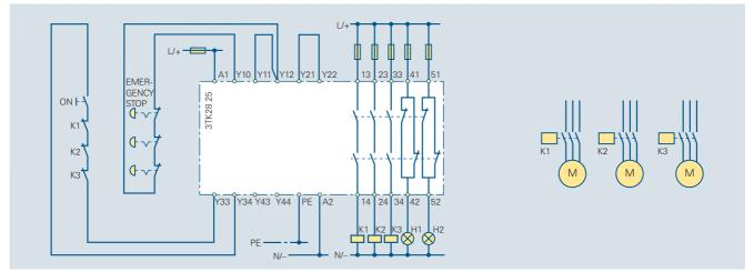
Fig. 7/13 3TK28 25 EMERGENCY STOP, Category 2, single-channel, according to EN 954-1, monitored start
