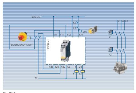
Fig. 7/48 SIGUARD 3TK2841, EMERGENCY STOP, Category 4 acc. to EN 954-1, two-channel, with feedback circuit, monitored start with "ON" button
