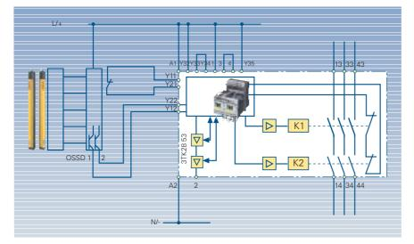
Fig. 7/73 The electronic basic 3TK2853 device with auxiliary contactors, cascading EMERGENCY STOP and protective door monitoring, 2-channel, Cat. 4 acc. to EN 954-1, SIL 3
