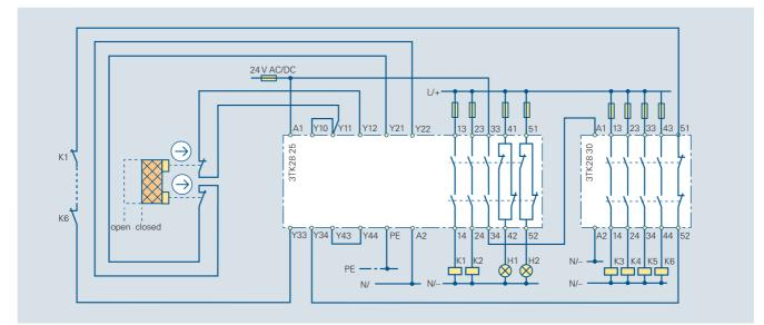
Fig. 7/30 3TK28 25 expanded by 3TK28 30 for protective door monitoring with 2 SIGUARD position switches, Category 4 acc. to EN 954-1, two-channel, with feedback circuit, autostart
