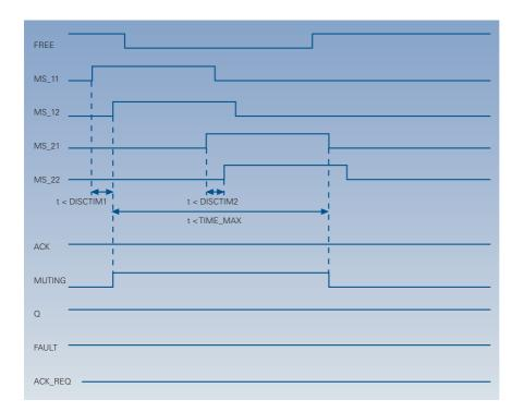
DISCTIM1 and DISCTIM2 are discrepancy times for sensor pairs 1 and 2.
