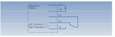
Example: Connection schematic for an anti-valent transmitter connected to an F-DI (2-from-2) through 2 channels
