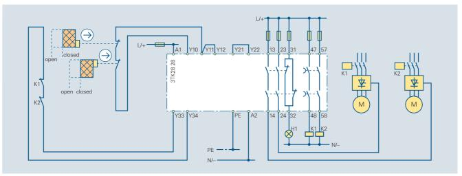
Fig. 7/28 3TK28 28 for protective door monitoring (2 protective doors are cascaded, each with 1 SIGUARD position switch), Stop Category 1, Category 2 acc. to EN 954-1, single-channel, with feedback circuit, autostart
