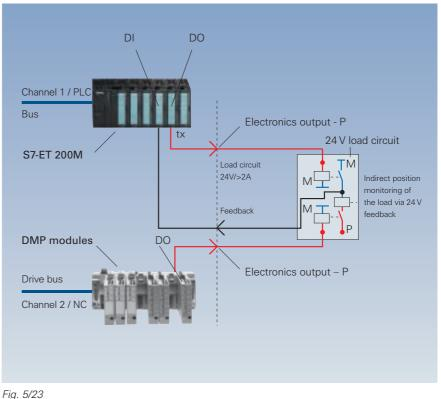
24 V load circuit – P/M switching with intermediate relay stage for > 2 A
