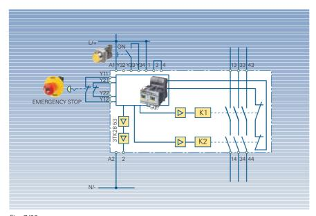
Fig. 7/66 The electronic basic 3TK2850 device with auxiliary contactors, EMERGENCY STOP, 2-channel, Category 4 acc. to EN 954-1 SIL 3
