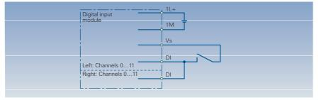
Example: Wiring schematic for a transmitter connected to an F-DI (2-from-2) through 1 channel)
