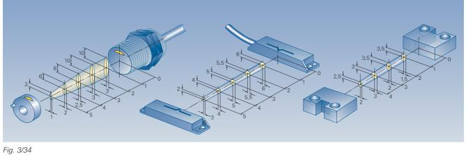
Enabling ranges of the SIGUARD magnetically-operated position switches 3SE6 605-.BA
