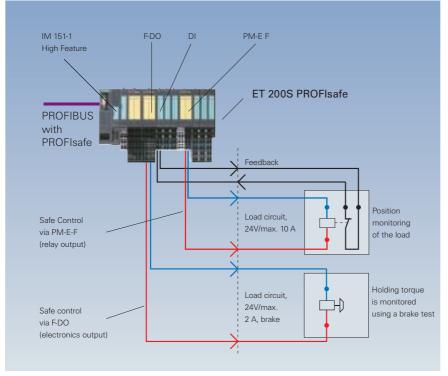
Fig. 5/27 24 V load circuit – P/M switching up to 2 A and up to 10 A
