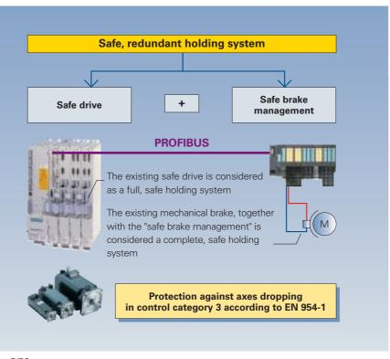
Fig. 5/30 Protection against vertical axes falling
