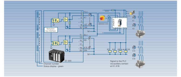
Fig. 7/52 SIGUARD 3TK2841, EMERGENCY STOP, Category 4 acc. to EN 954-1, in conjunction with operational control of a standard PLC (SIMATIC S7 300/ET200M) load current for each enable circuit, max. 2 A
