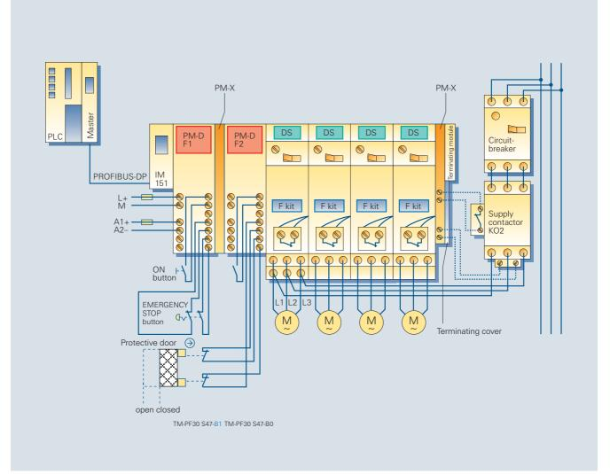
Fig. 7/86 EMERGENCY STOP combined with protective door
