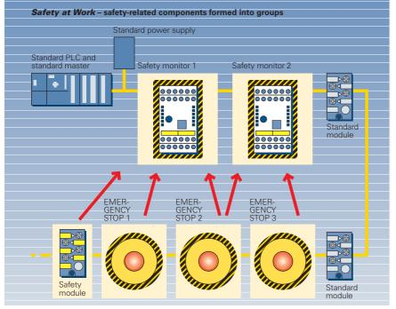
A PC is used to assign the safetyrelated slaves to the Safety Monitors.
