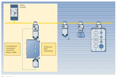
Fig. 2/16 Protective door monitoring, Category 3/4 with safety AS-Interface adapter and additional spur
