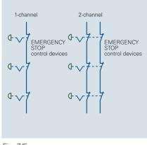
Fig. 7/5 Several EMERGENCY STOP control devices
