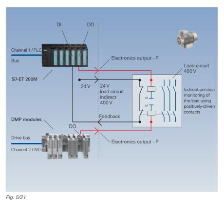
400 V load circuit – P/P switching – example of a standard asynchronous motor
