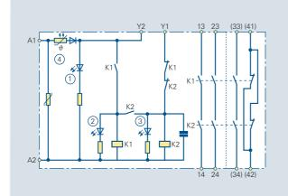
Fig. 7/9 Internal circuit diagram of the 3TK28 21/24
