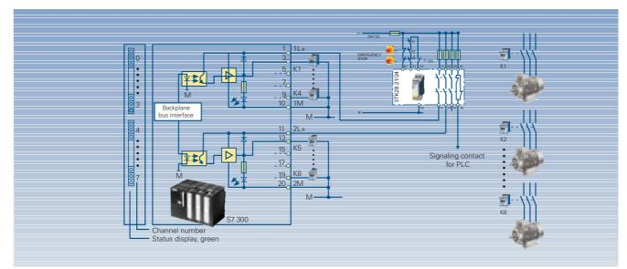
Fig. 7/21 EMERGENCY OFF, Category 2 acc. to EN954-1, 3TK2821 in conjunction with operational control of a standard PLC (SIMATIC S7-300/ET200M), load current, max. 5 A per output group (8 digital outputs)
