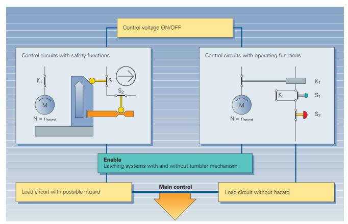
Fig. 2 General configuration of a machine control system (DIN VDE 0113/11.98)
