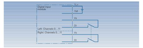
Example: Wiring schematic for a transmitter connected to an F-DI (2-from-2) through 2 channels)
