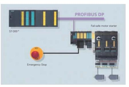
Fig. 4/10 Direct control of motor starters through ET 200S PROFIsafe
