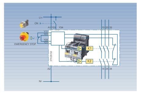
Fig. 7/64 The electronic basic 3TK2850 device with auxiliary contactors, EMERGENCY STOP, 1-channel, with additional ON button, Category 2 acc. to EN 954-1
