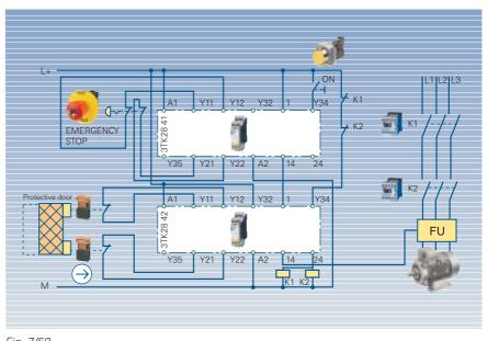
Fig. 7/58 SIGUARD 3TK2841, cascaded with 3TK2842 for EMERGENCY STOP, 2-channel, monitored start with ON button and protective door monitoring, 2-channel, autostart, Category 4 acc. to EN 954-1
