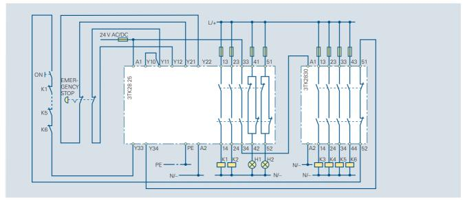
Fig. 7/18 3TK28 25 expanded by 3TK28 30 for EMERGENCY STOP, Category 4 acc. to EN 954-1, two-channel cc. to EN 954-1, monitored start
