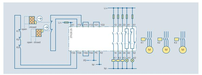
Fig. 7/26 3TK28 25 for protective door monitoring (2 protective doors are cascaded, each with 1 SIGUARD position switch), autostart, Category 2 acc. to EN 954-1, single-channel, with feedback circuit
