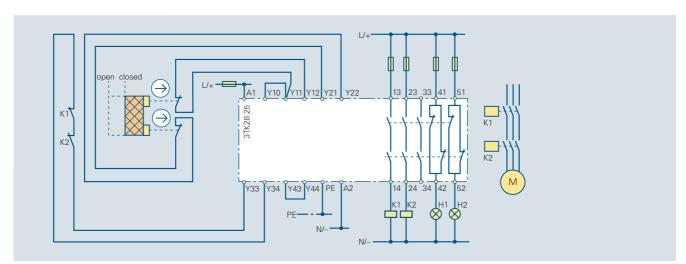
Fig. 7/27 3TK28 25 for protective door monitoring with 2 SIGUARD position switches, autostart, Category 4 acc. to EN 954-1, two-channel, with feedback circuit
