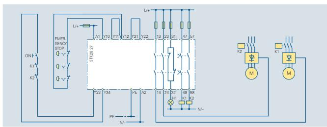
Fig. 7/15 3TK28 27 EMERGENCY STOP, Category 2, single-channel, according to EN 954-1, monitored start
