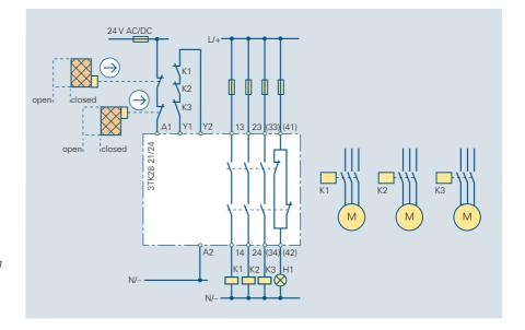
Fig. 7/22 3TK28 21/24 for protective door monitoring (2 protective doors are cascaded each with 1 SIGUARD position switch), Category 2 acc. to EN 954-1, single-channel, with feedback circuit, autostart
