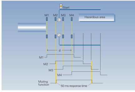
Muting sensors can be pushbuttons, proximity switches, light barriers, and limit switches etc., which do not have to be fail-safe. The redundant fault monitoring is realized using the muting evaluation unit in compliance with the requirements for Category 4 according to EN 954-1. If the muting sensors are actuated in the correct sequence (in time), the muting evaluation unit switches into the muting mode and bypasses the fail-safe outputs of the light curtain.
