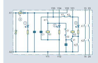
Fig. 7/7 Internal circuit diagram of the 3TK28 23
