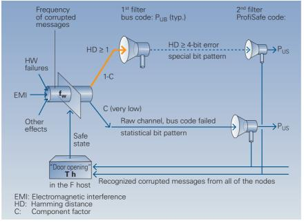
bus such as PROFIBUS. Thus, a mechanism was created which guarantees that all of the SIL stages are maintained over the lifetime of a distributed safety-related automation solution, independent of the components and configuration used: A patented SIL Monitor, which is implemented in the software.
