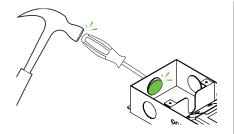
a. Use punch and hammer to loosen K/O.
