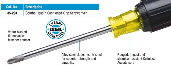
Different sizes of Combination Fasteners mean using different tools, right? Wrong! The Combo Head™ was designed to fit snuggly into multiple sizes of Combo Screws, eliminating the need to buy more bulky tools. Among the competition, the IDEAL Combo Head<sup>™</sup> tip features the most touch points, minimizing cam-out and stripping. See and feel the difference for yourself!
