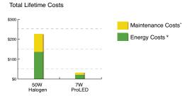
Maintenance costs based on 15 minutes to replace the lamp at \$40 per hr over the life of the ProLED lamp.
