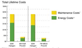
Maintenance costs based on 15 minutes to replace the lamp at \$40 per hr over the life of the ProLED lamp. YEnergy costs based on \$0.11 kWh over 40,000 hour life.
