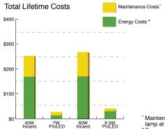
Maintenance costs based on 15 minutes to replace the lamp at \$40 per/hr over the life of the ProLED lamp.
