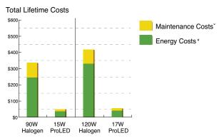
Maintenance costs based on 15 minutes to replace the lamp at \$40 per hr over the life of the ProLED lamp.
