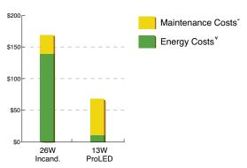
Maintenance costs based on 15 minutes to replace the lamp at \$40 per hr over the life of the ProLED lamp. Y Energy costs based on \$0.11 kWh over 40,000 hour life.
