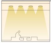
Lighting throughout an area which produces general illumination. The appropriate Halo recessed fixtures are available to provide patterns of light distribution for this purpose. These units direct light in specific patterns to illuminate areas without drawing attention to the fixtures themselves.
