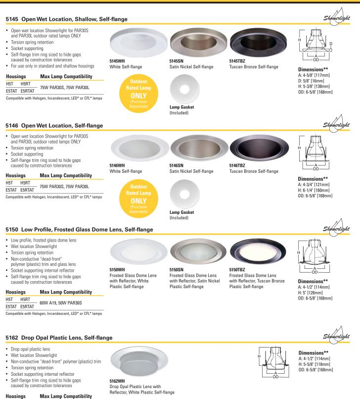
\*UL1993 listed LED & CFL equivalent lamps permitted. Consult lamp manufacturer for conditions of use. Eaton does not warranty the lamp.
