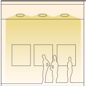
Lighting of vertical surfaces defines form, space and texture. It can visually increase the apparent size of a room while improving visual comfort. Halo has skillfully engineered fixtures designed to direct a spread of illumination on these surfaces. Halo fixtures may be selected based on the size of the space, the level of illumination and intensity desired, energy efficiency and controllability.
