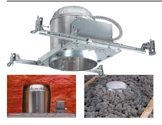
Insulated Ceiling type (IC) rated luminaires are tested to UL 1598 standards for installation with blown-in or batting-type dry insulation materials. This allows the insulation layer to remain unbroken and prevent heating and air conditioning losses. These housings are also equipped with thermal protectors to guard against overlamping by cycling the lamp off and on until the problem is corrected.
