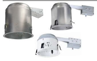
Remodel housings simplify installation when fixtures need to be added to existing ceilings. They can be installed from below in existing ceilings by cutting a precise hole, bringing power to the fixture and installing the housing. The spring clips or speed clamps lock the fixture in place. The integral thermal protector provides positive protection against overlamping. Housings are available in Insulated Ceiling (IC), Non-Insulated Ceiling (Non-IC), Air-Tite (AT) and shallow models.
