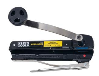
The Klein Tools BX and Armored Cable Cutter is simple to use. It easily cuts 3/8-Inch flexible conduit and #10, 12, and 14 armored cables with a couple of turns of the handle. Extra blades can be stored in the handle for convenience.
