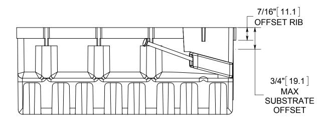
1.) BOX MATERIAL: FIBERGLASS REINFORCED POLYESTER, NAIL MATERIAL: PLATED CARBON STEEL, SPEED KLAMP MATERIAL: PVC
