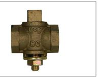
Bronze body and plug manually operated low pressure natural or propane gas valve for use indoors on house piping system between the meter oulet and the inlet connection of the gas appliance at ambient temperatures of 32 to 125 degrees Fahrenheit.
