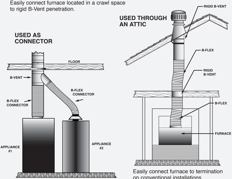
Make direct connection from one or both appliances to common B-Vent.
