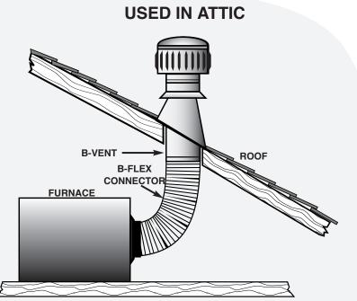
Make quick connection from attic furnace to rigid B-Vent penetration.
