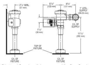
Side Mount Operator unit shown on an existing Sloan Regal Model 180 or 186 Urinal Flushometer
