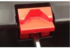
To remove a damaged locker system, flip tote over on the side and approach tote from the bottom of base. Insert a large flat blade screwdriver in middle of locking carriage as shown. Lightly pry carriage upward out of base opening. Remove and discard old locking carriage.
