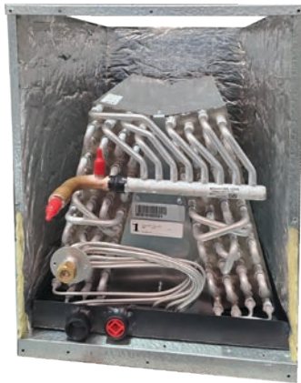
Unit shown with service panels removed. Representative photo only. Some models may vary in appearance. Duct opening dimensions can be ascertained by subtracting 1 1/2" for top opening width/depth, 3/4" for bottom opening.
