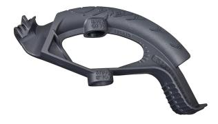
Klein Tools Conduit Bender Head is designed to handle thin wall EMT up to 1-Inch and rigid IMC up to 3/4-Inch thick. Made from Iron with Klein's advanced casting process for the ultimate in core strength and durability. This head works with the Klein Handle (Cat. No. 51428) which is sold separately.
