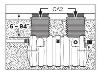
DO NOT COMPACT BACKFILL MECHANICALLY Compact by hand only
