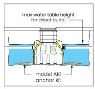
risk areas include but are not limited to tidal surge areas, floodplains and areas that receive storm water. Great Basin™ models that are direct buried in high water table scenarios must be installed with an anchor kit. Model GB-75 uses model AK1 anchor kit.
