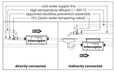
If water is entering the interceptor at excessive temperature (over 150° F), a drain water tempering valve (DTV) and approved backflow prevention assembly must be installed. Most state and local plumbing codes prohibit water above 150° F being discharged into the sanitary sewer. Water above 150° F will weaken or deform PVC Schedule 40 pipe, poly drainage fixtures like interceptors and erode the coating of cast iron (leading to eventual failure).
