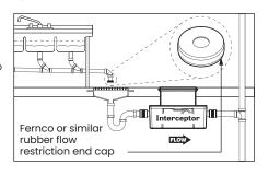
See drawing for guidance. For detailed guidance on indirect connections, go to:
