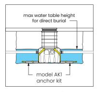
At risk areas include but are not limited to tidal surge areas, floodplains and areas that receive storm water. Great Basin™ models that are direct buried in high water table scenarios must be installed with an anchor kit. Model GB-50 uses model AKI anchor kit.
