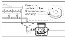
done by installing a valve or flow restriction cap on the sink piping that discharges into the drain. See drawing for guidance. For detailed guidance on indirect connections, go to:
