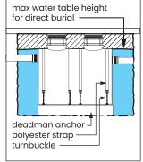
water. Great Basin<sup>™</sup> models that are direct buried in high water table scenarios must be installed with an anchor kit. Model GB-1000 uses model AK3 anchor kit for use with deadmen anchors.
