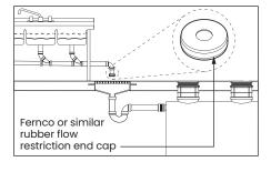
installing a valve or flow restriction cap on the sink piping that discharges into the drain. See drawing for guidance. For detailed guidance on indirect connections, go to: webtools.schierproducts.com/Technical\_Data/Indirect\_Connections.pdf
