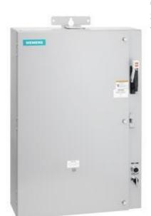
Pump control panel, Size 4, Three phase full voltage, Solid-state overload relay, OLR amp range 50-200A, 220-240/440-480VAC 60Hz coil, Standard type contactor, 200A fusible disconnect, 200A/250V fuse clip, HOA Sel Sw. & Start P.B., Enclosure NEMA type 3/3R, Weather proof outdoor use
