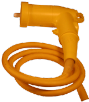
Figure 28. Grounding elbow is molded of bright yellow EPDM rubber for easy identification. Six-foot flexible copper, 600 volt insulated cable is available in 1/0 or 2/0. Elbow is fully rated for fault close to ensure operator safety.
