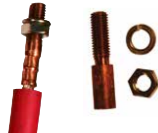
Figure 6. Ferrule installed on cable.
