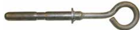
Figure 32. Test probe has an eye for easy hotstick handling. It allows electrical access to the bushing contacts so that circuit condition can be confirmed using appropriate test equipment. It should not be used for grounding because it has no fault-close rating.
