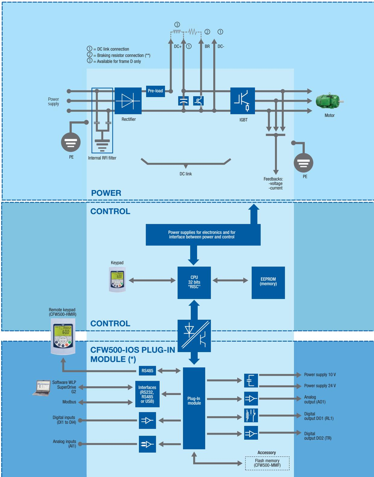
Notes: (\*) The number of inputs and outputs (analog and digital), as well as other resources, may vary according to the used plug-in module. For further information, refer to the CFW500 user manual.
