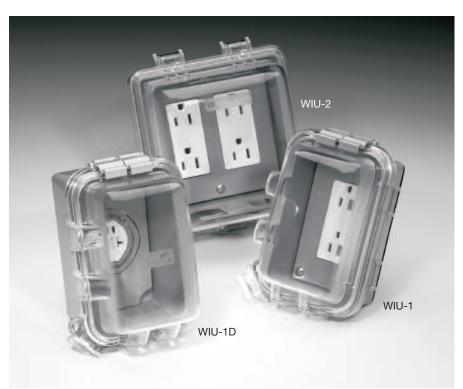
Each Single-Gang and Extra Deep cover comes standard with three inserts for a total of 16 different configurations. Included are duplex and decorator inserts, plus a single receptacle/toggle insert with easy punch-outs that can accommodate 5 sizes of receptacles from 1.25" to 2.125".
