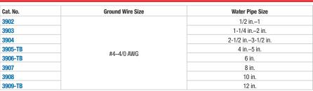
Material: Steel U-bolt and nut c/w bronzed aluminum cap and crossbar cadmium plated plus gold chromate finish.
