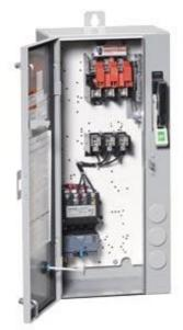
Non-reversing motor starter Size 0 Three phase full voltage Solidstate overload relay OLRelay amp range 3-12A 24VAC 50-60HZ coil Combination type 30Amp fusible disconnect 30 Amp /600V fuse clip Enclosure NEMA type 4/12 Water/dust tight weather proof Standard width enclosure
