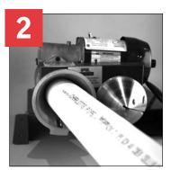
Sand outside corner of pipe around entire diameter using sanding sponge for a minimum of 20 seconds.
