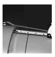
To ensure joint integrity, once insertion is complete, the pulling tool can be used to hold the joint in place during set time and also to ensure that the pipe does not back out.
