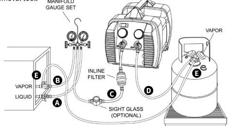
2. Close both valves on the Manifold Gauge Set. Open both valves on the G5Twin, open both valves on the Recovery Cylinder, and open the VCRT ball valves at the AC/R System access ports (if equipped).
