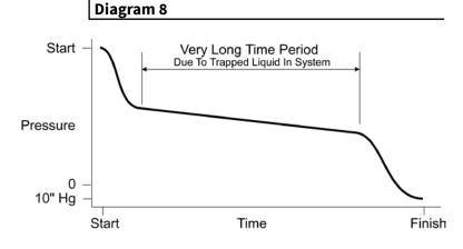
Pretty soon, the recovery machine is only receiving a <u>reduced flow of vapor</u> that is now <u>picking up ambient</u> <u>heat</u> and <u>adding it to the heat of compression</u>. All of this heat is sent along to the recovery cylinder, quickly <u>raising the recovery cylinder temperature</u>.
