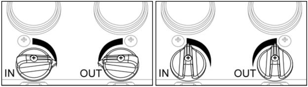
**Horizontal Knobs: Valves Closed**
