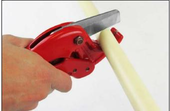
Be careful not to split the pipe if using a ratchet-type cutter, especially in temperatures below 50°F. If any damage or cracking is evident, cut off at least 2" of the pipe beyond any visible crack.
