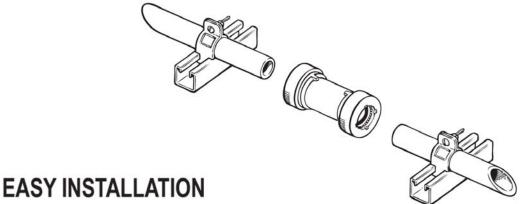
STEP 1 Cut pipe square. Deburr and bevel.
