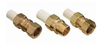
Standard compression fittings with brass or plastic ferrules can be used. However, PTFE tape should be applied over the brass ferrule to compensate for the dissimilar thermal expansion rates between the brass and CPVC.
